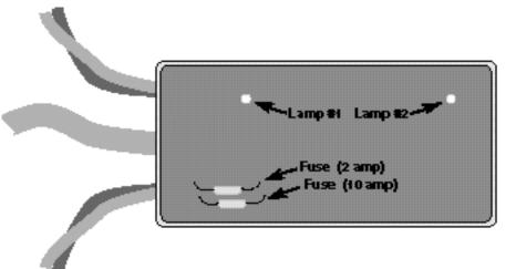
indicators which are labeled Lamp #1 and Lamp #2 will be used in the system fault diagnosis steps that follow
