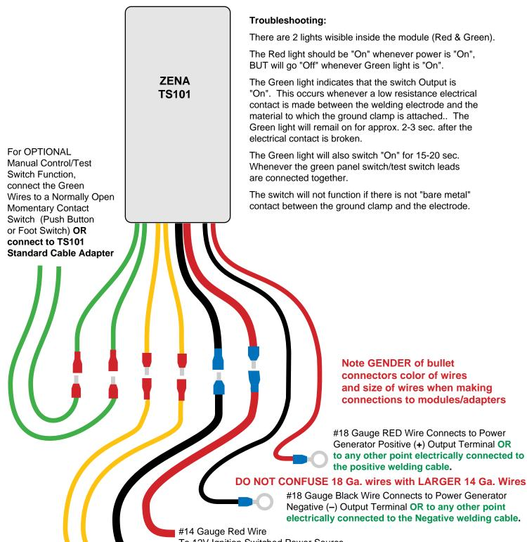
To 12V Ignition Switched Power Source **DO NOT CONFUSE 14 Ga. wires with SMALLER 18 Ga. Wires** #14 Gauge Black Wire Chassis Ground
