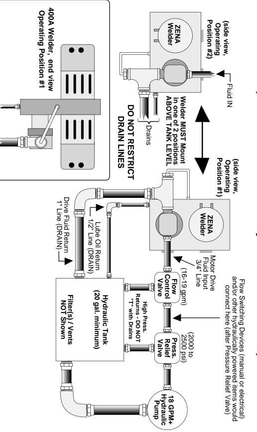
(Welder Drive Box ABOVE Hydraulic Reservoir Tank) Standard, Gravity Lube Oil Return Version Typical ZENA<sup>™</sup> Hydraulic Welder Hookup
